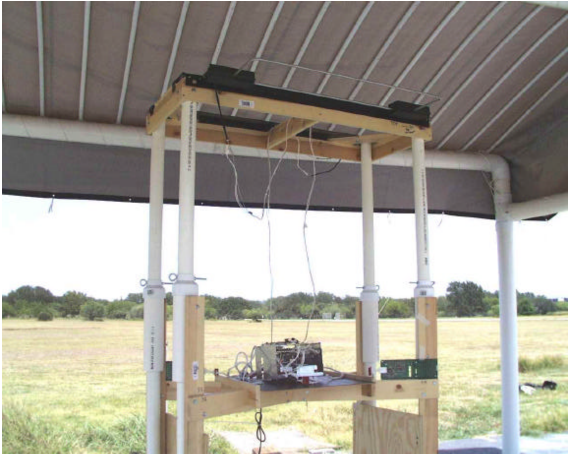
Radiated Emissions OATS Test Setup – Encore Configuration
