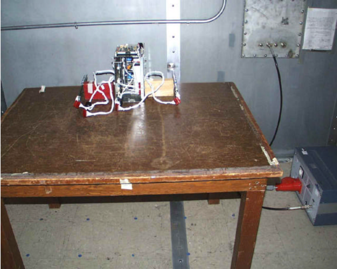
Conducted Emissions Test Setup – Encore Configuration
