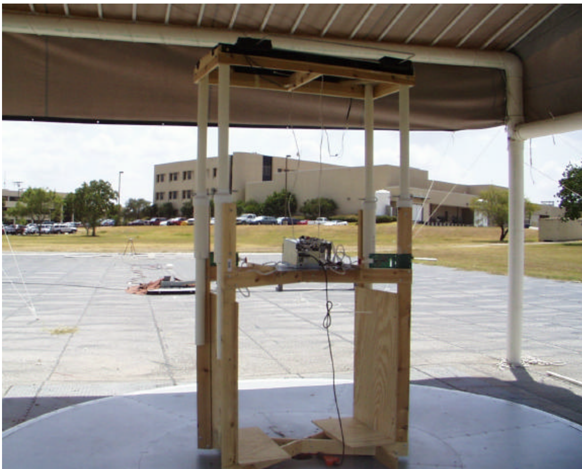
Radiated Emissions OATS Test Setup – Encore Configuration
