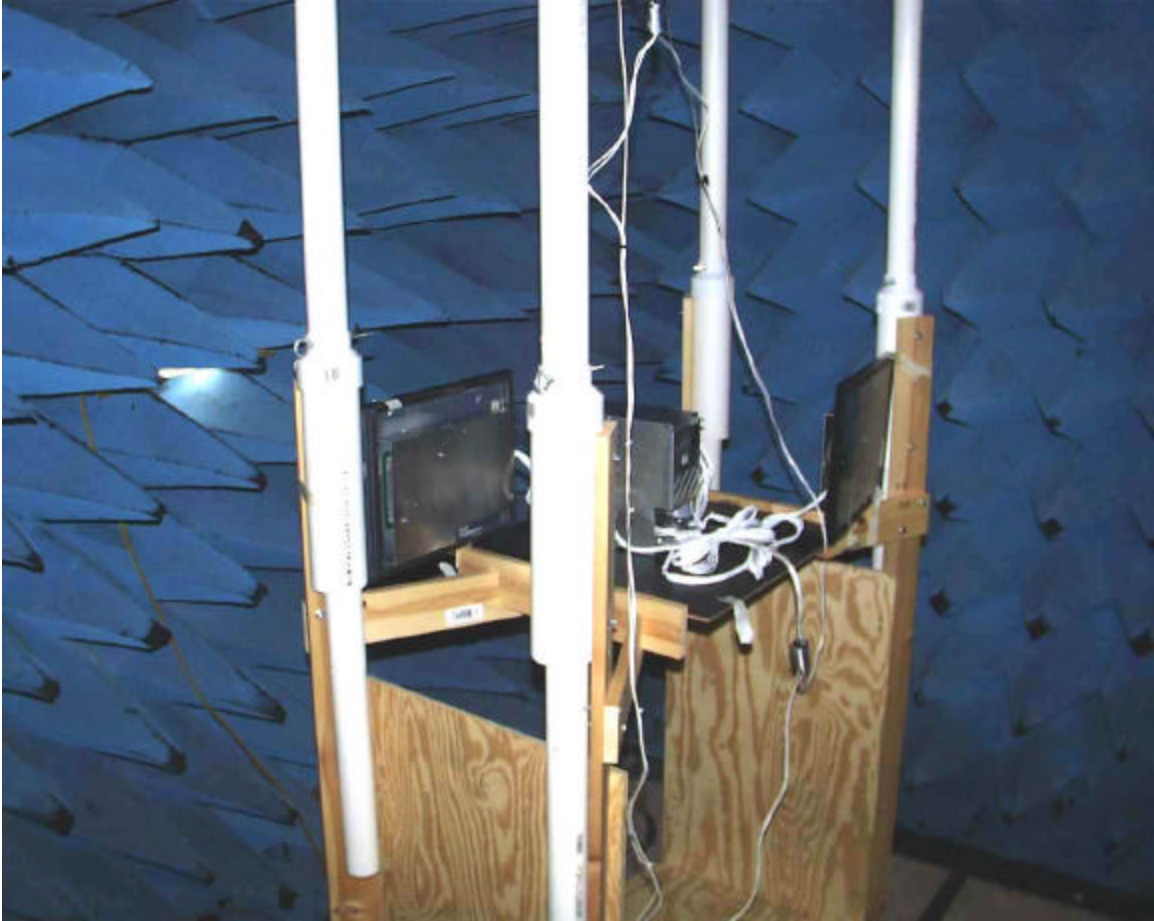
Radiated Emissions Pre-scan (Anechoic) Test Setup – Advantage Configuration
