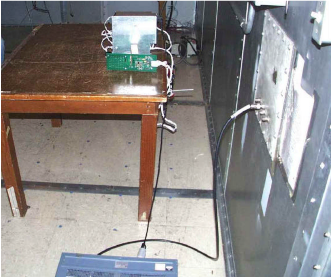
Conducted Emissions Test Setup – Encore Configuration
