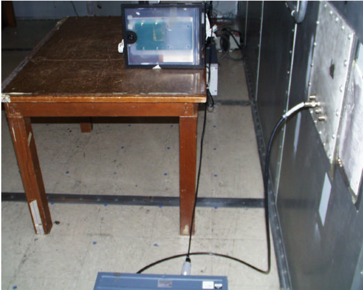
Conducted Emissions Test Setup – Advantage Configuration
