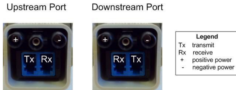
Figure 4: Fibre orientation of Upstream and Downstream ports
