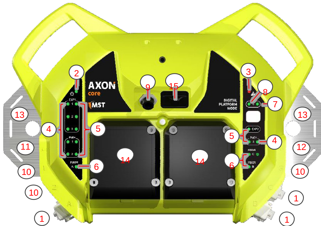
Figure 2: AXON Core layout
