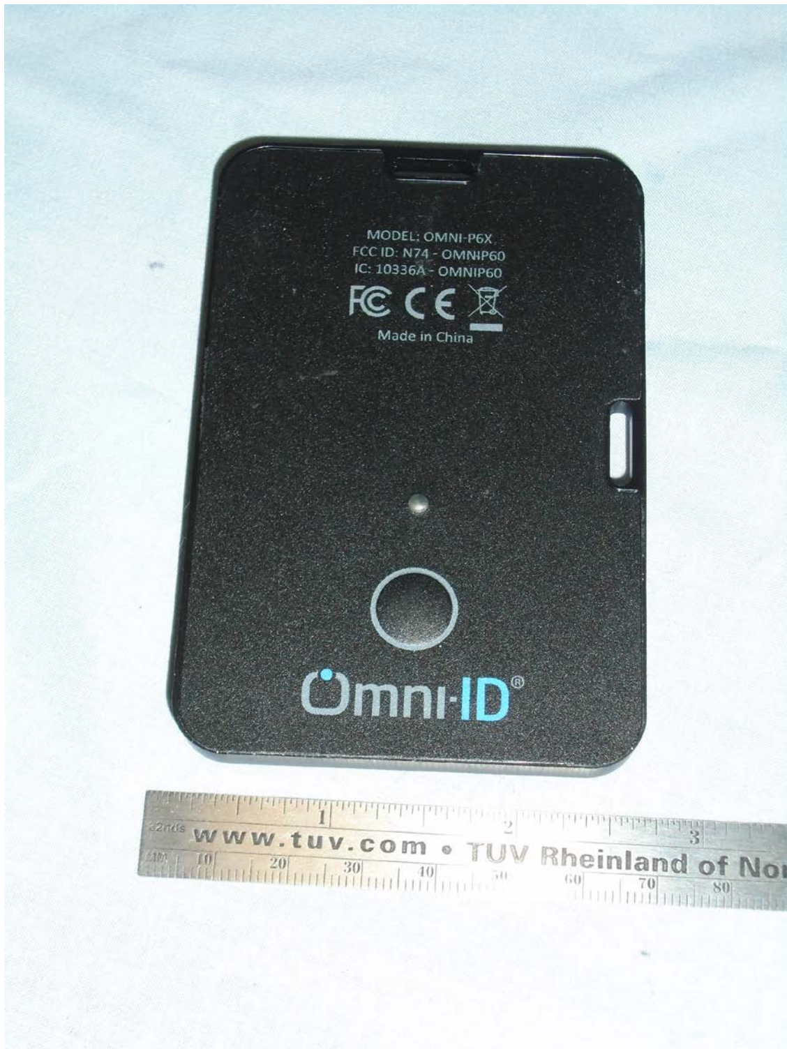
Figure 1: View of Label Location on EUT Note: The “P6X” will be replaced with a P60 or P65
