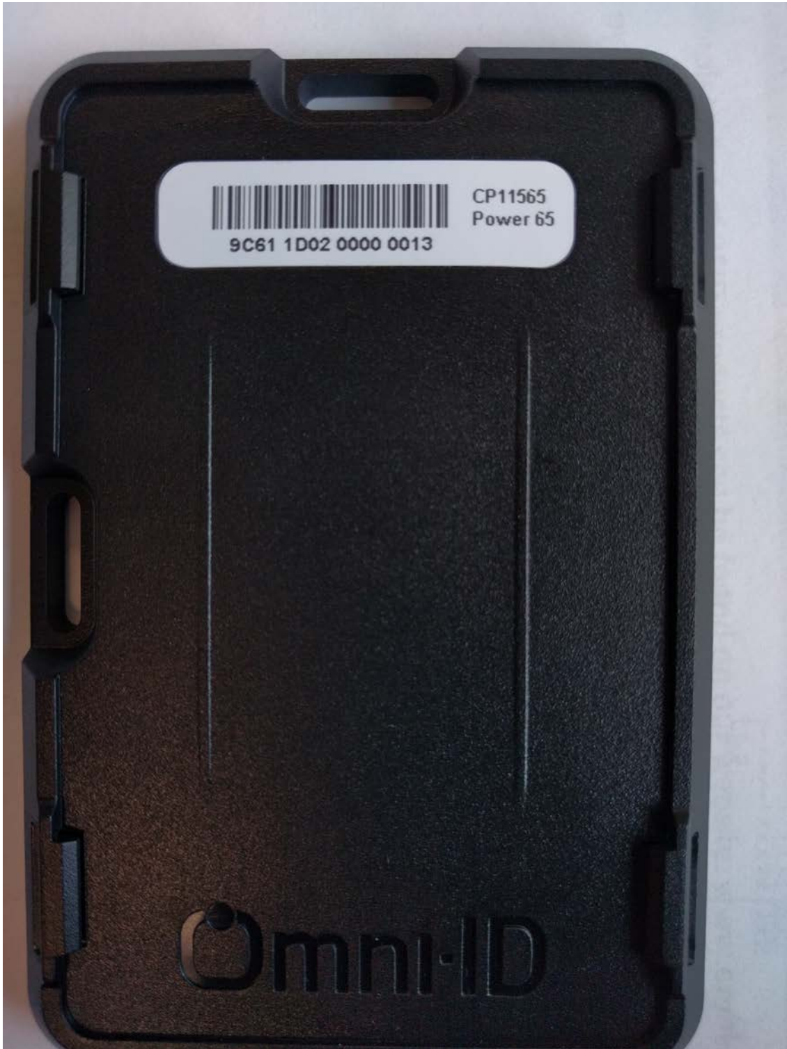
Figure 2: View of Label Location for Part Number and MAC ID inside the EUT Case for the OMNI-P65 Note: The Label location is identical for the OMNI-P60
