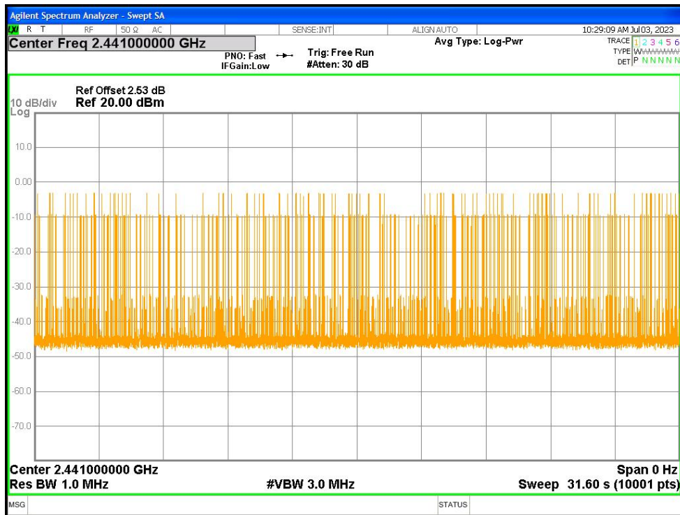
Dwell NVNT 3-DH5 2441MHz Ant1 One Burst
