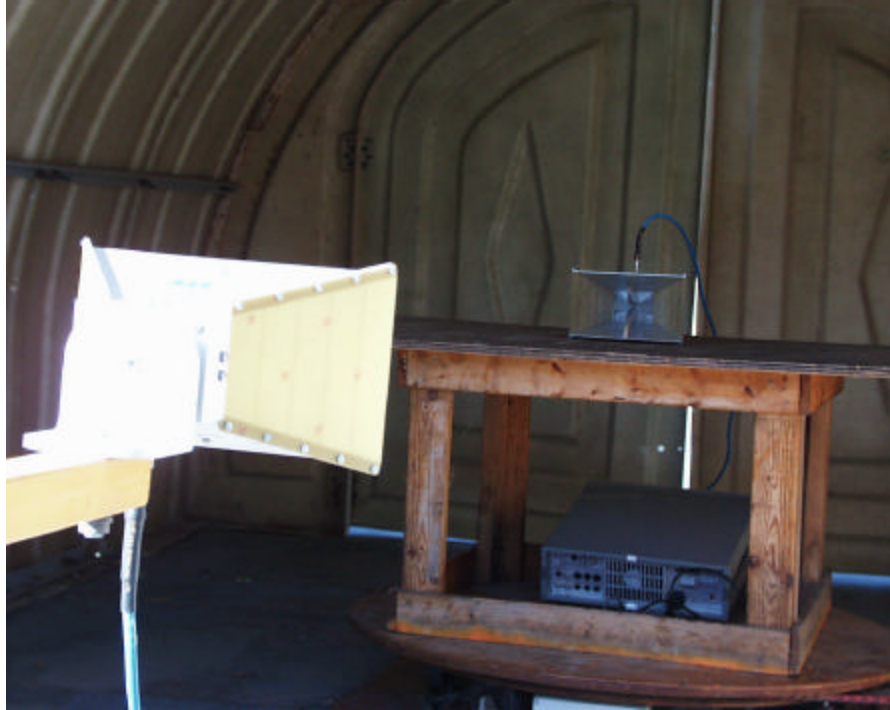
Substitution Method @ 1900 MHz
