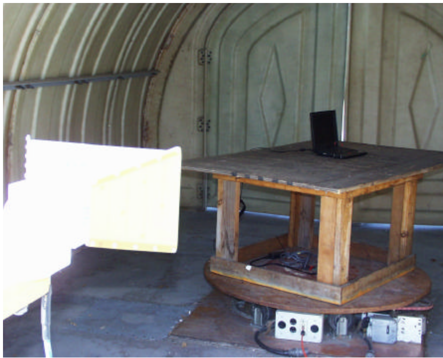
ERP Setup @ 1900 MHz
