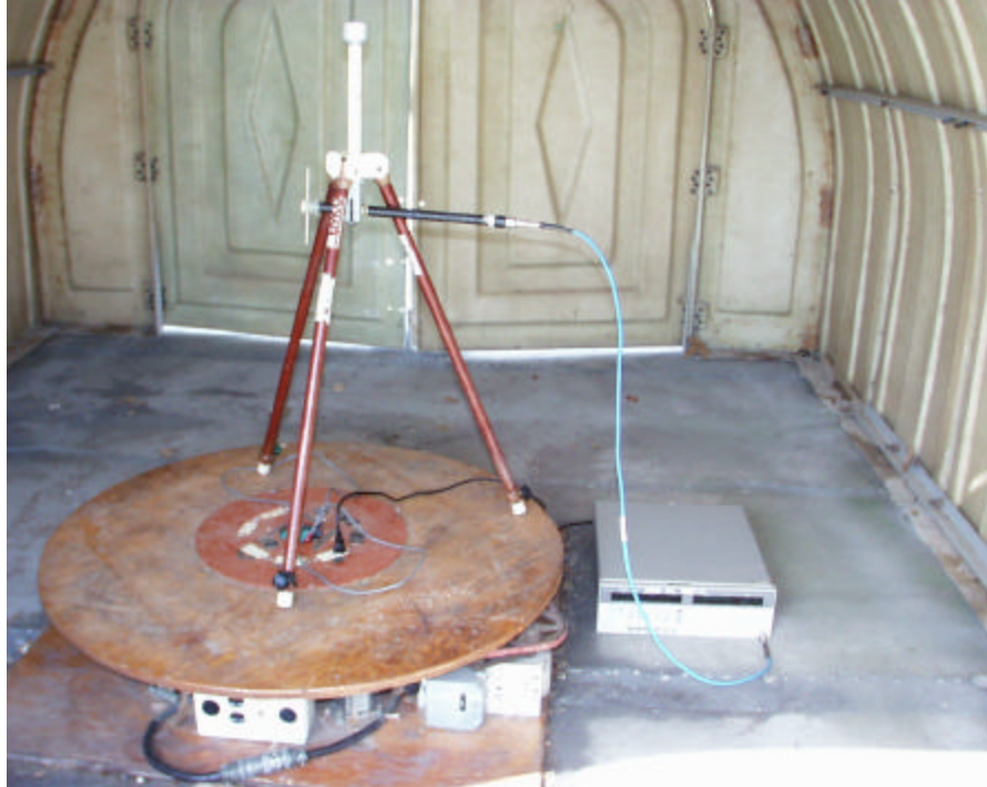
Substitution Method @ 800 MHz
