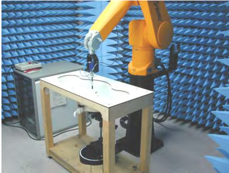
Fig.1 Photograph of the SAR measurement System
