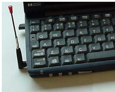
Figure 5-1: Proper positioning of the AirCard antenna
