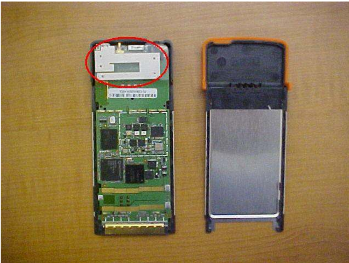
3) AC875 case opened with antenna circled in red.
