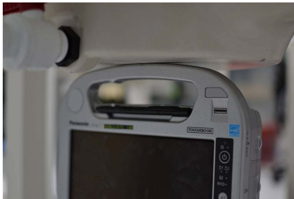
SAR Test Setup Photo 2 – Top Edge at 0.0 cm
