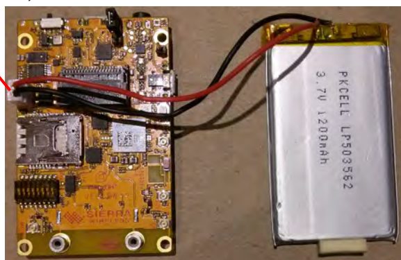
Figure 3-5: mangOH Yellow With Rechargeable Battery Connected
