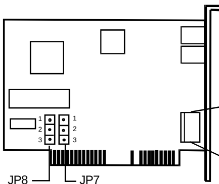
Figure 2-4 COM/IRQ Jumper Location for Model I601
