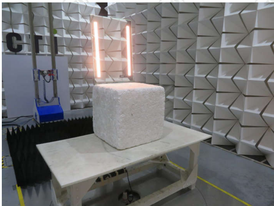
Radiated spurious emission Test Setup-3(Above 1GHz)
