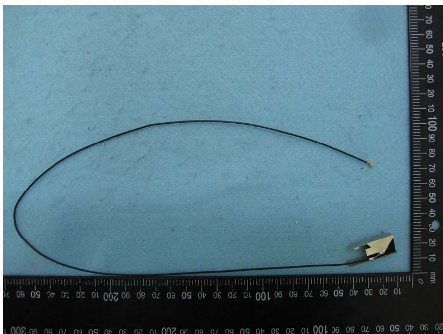
PIFA Antenna (Only for Bluetooth Function)
