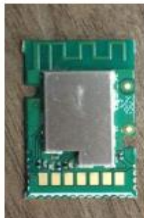
Drawing 2-2 Real Module Drawing for LSD4RF0436-10D0
