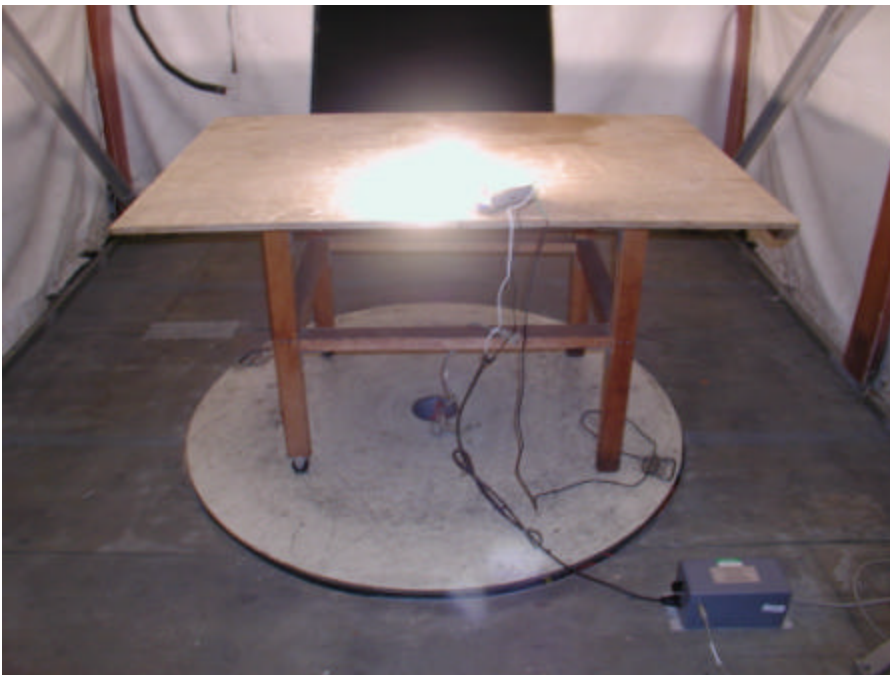
CFM32W Conducted Emission Photograph – Rear View
