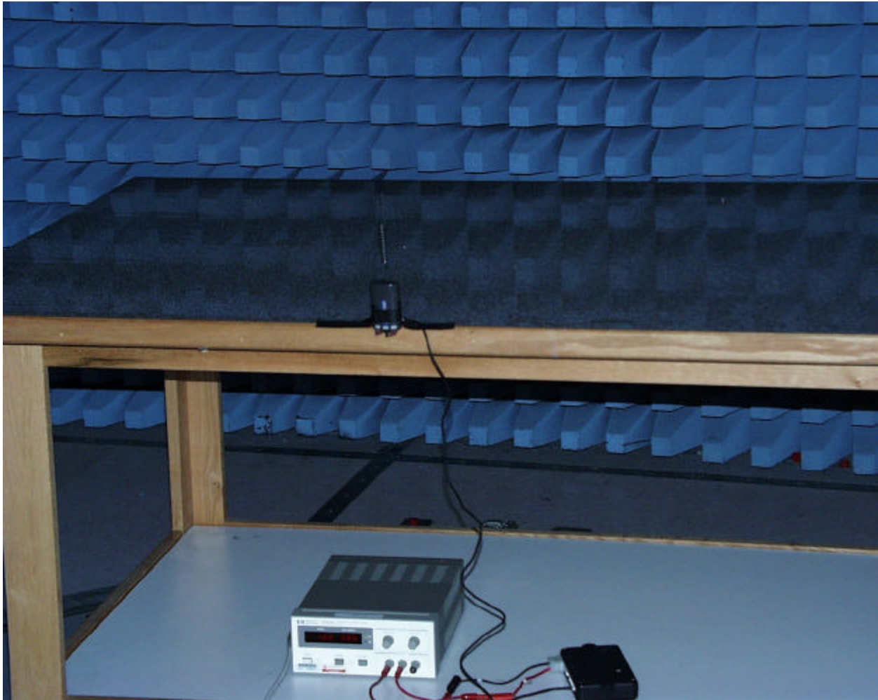
Front View of Radiated Test Setup
