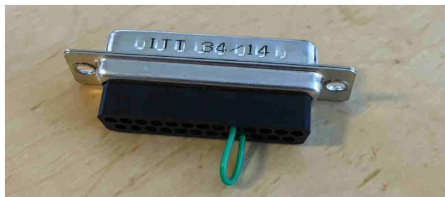
Fig. 7.1 25-pin D-SUB male connector with one wire
