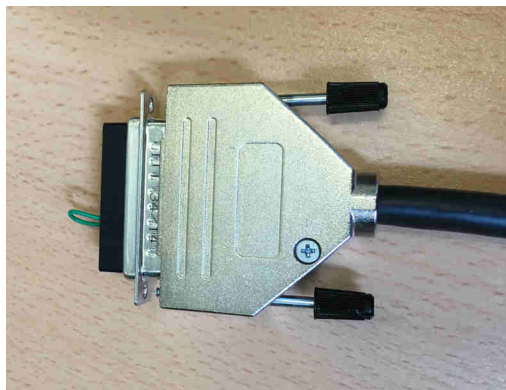
Fig. 7.5 W8 connected to 25-pin D-SUB male connector
