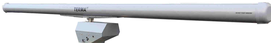
Fig. 6.1 Compact antenna with fixed turning unit
