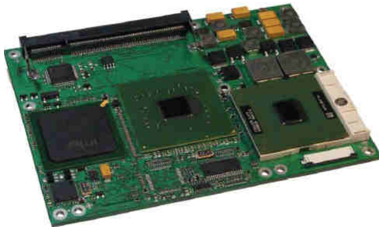
Fig. 4.20 PC Controller Board
