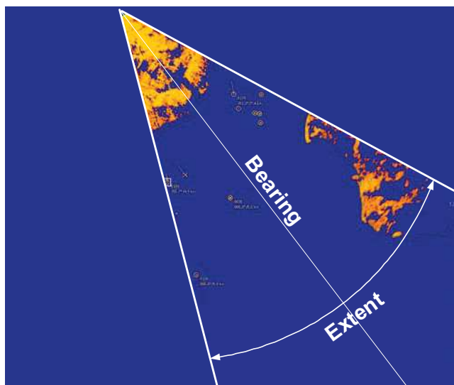
Fig. 5.13 Sector Bearing and Width
