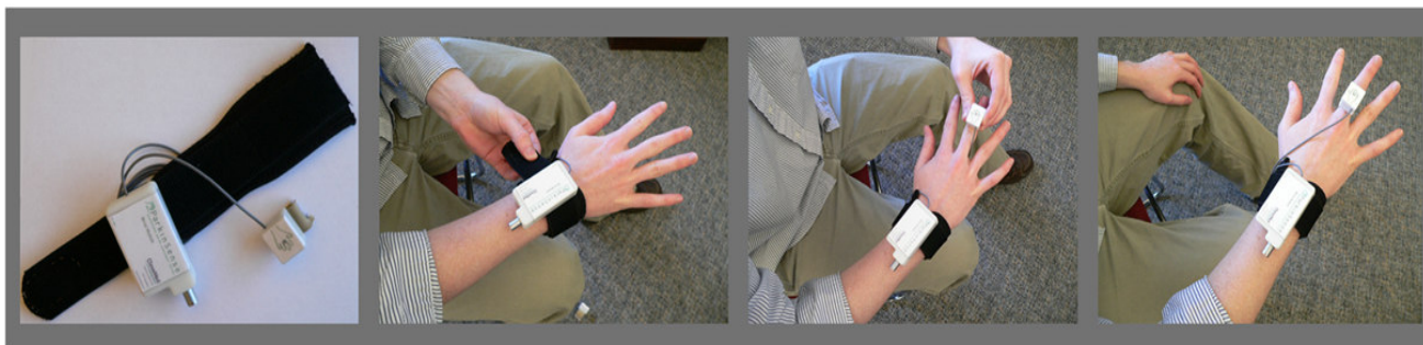
Figures 2 – 5. From left to right. 2Add pictures here to show setup. Fig 2. Wrist band alone, Fig 3. Sliding over the finger, Fig 4. Sliding over wrist band. Fig 5. Complete System.
