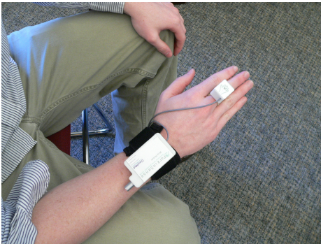
Figure 1. The user unit is worn by the subject and consists of finger and wrist worn components.
