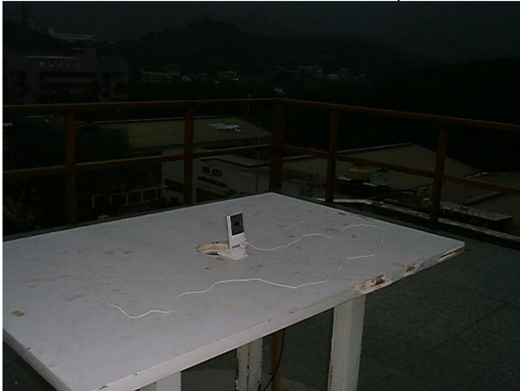
Measurement of Radiated Emission Test Set Up
