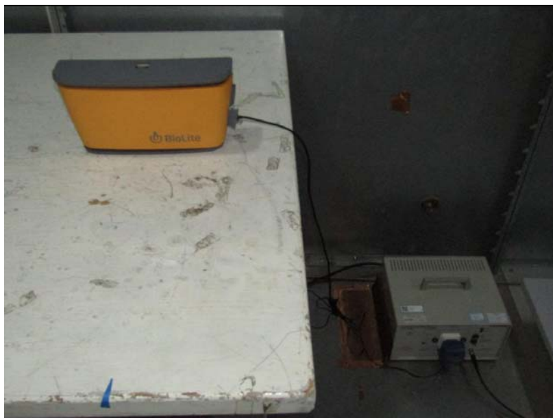
Measurement of Conducted Emission Test Set Up
