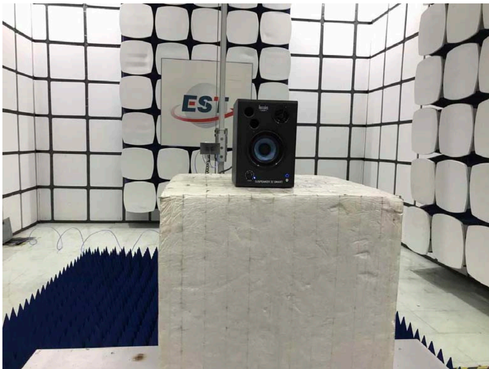
Radiated test: Above 1GHz
