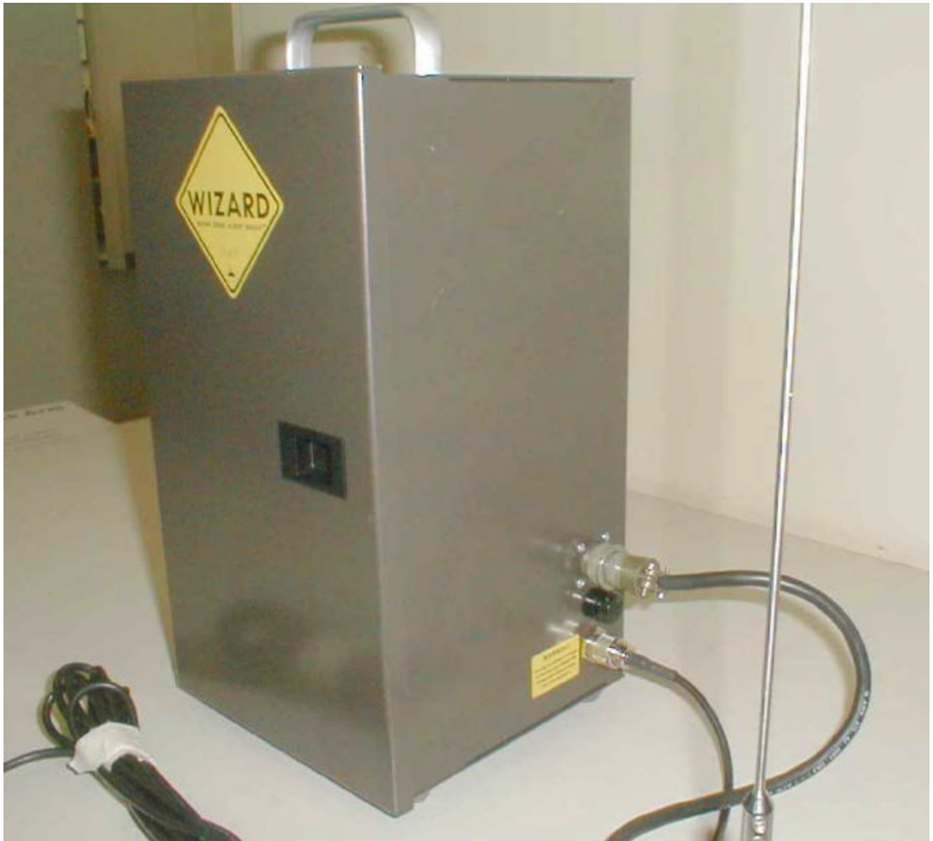
Side View, Fuse Holder, Connectors: Power and Antenna
