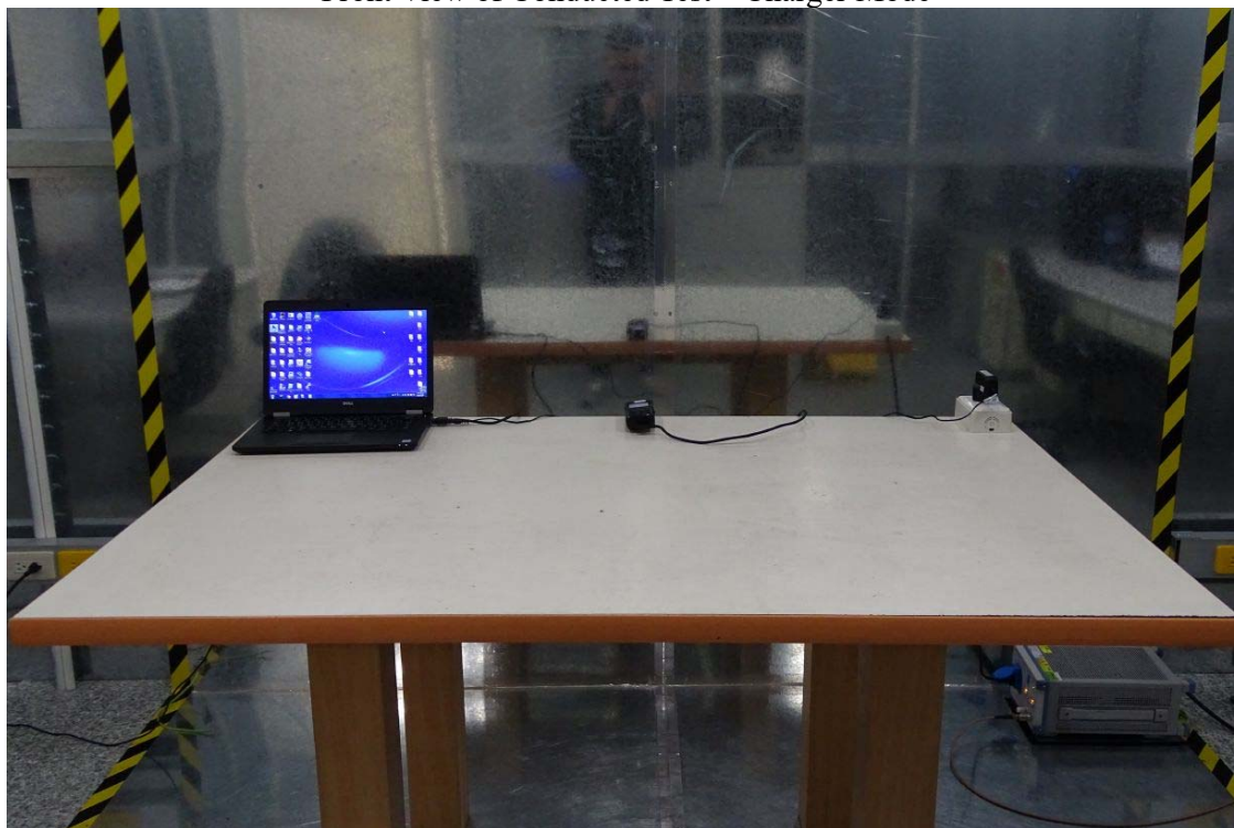
Front View of Conducted Test – Charger Mode
