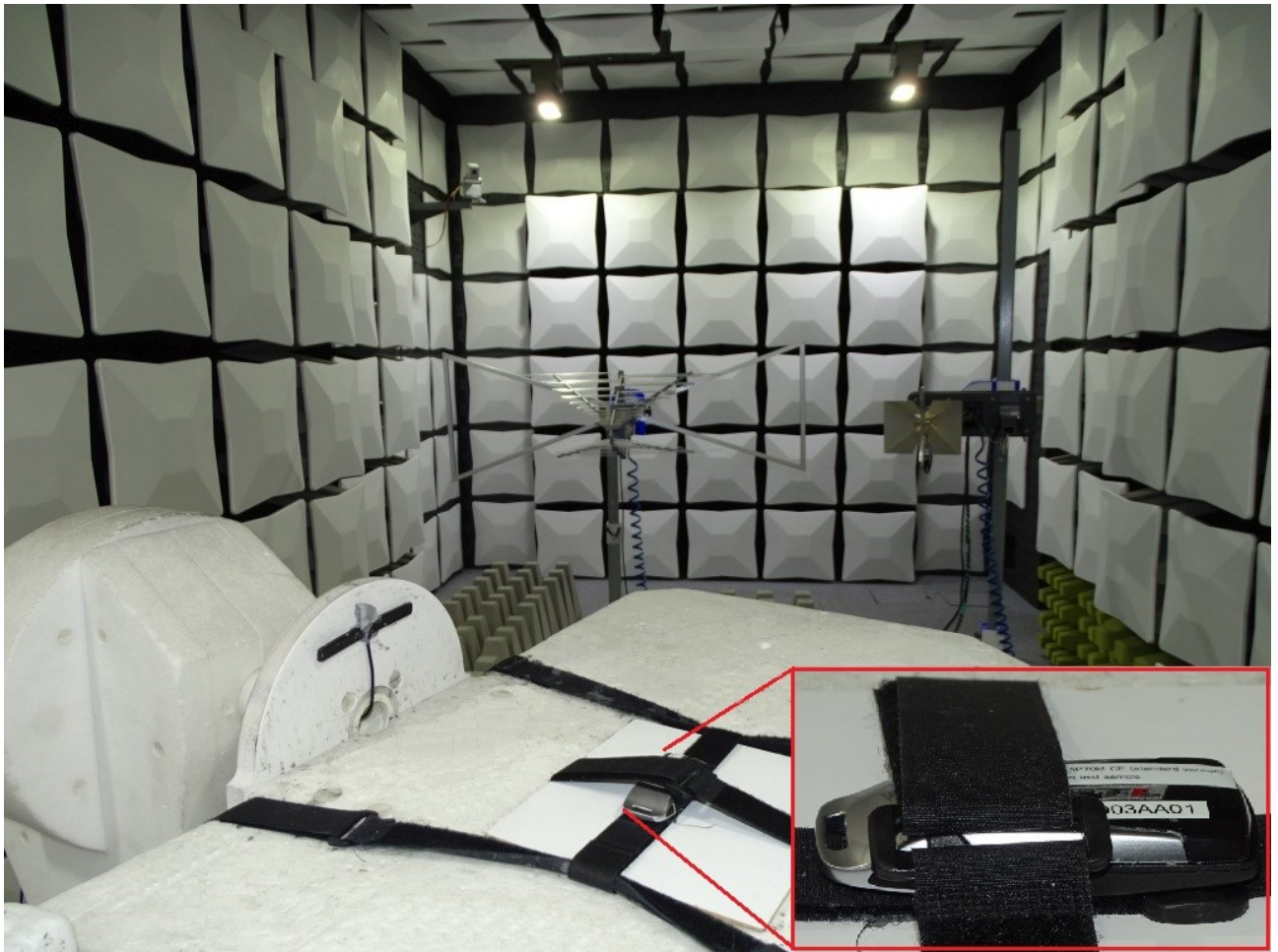
Photo 3: Test setup for radiated measurements (Enclosure, fully-anechoic chamber, 1-6 GHz intentional radiator §15, ANSI C63.10)
