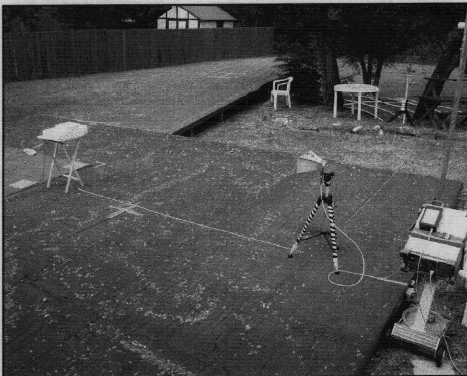
Photo 22: PROX-V, Maximum Emission Verification on 3 m OATS
