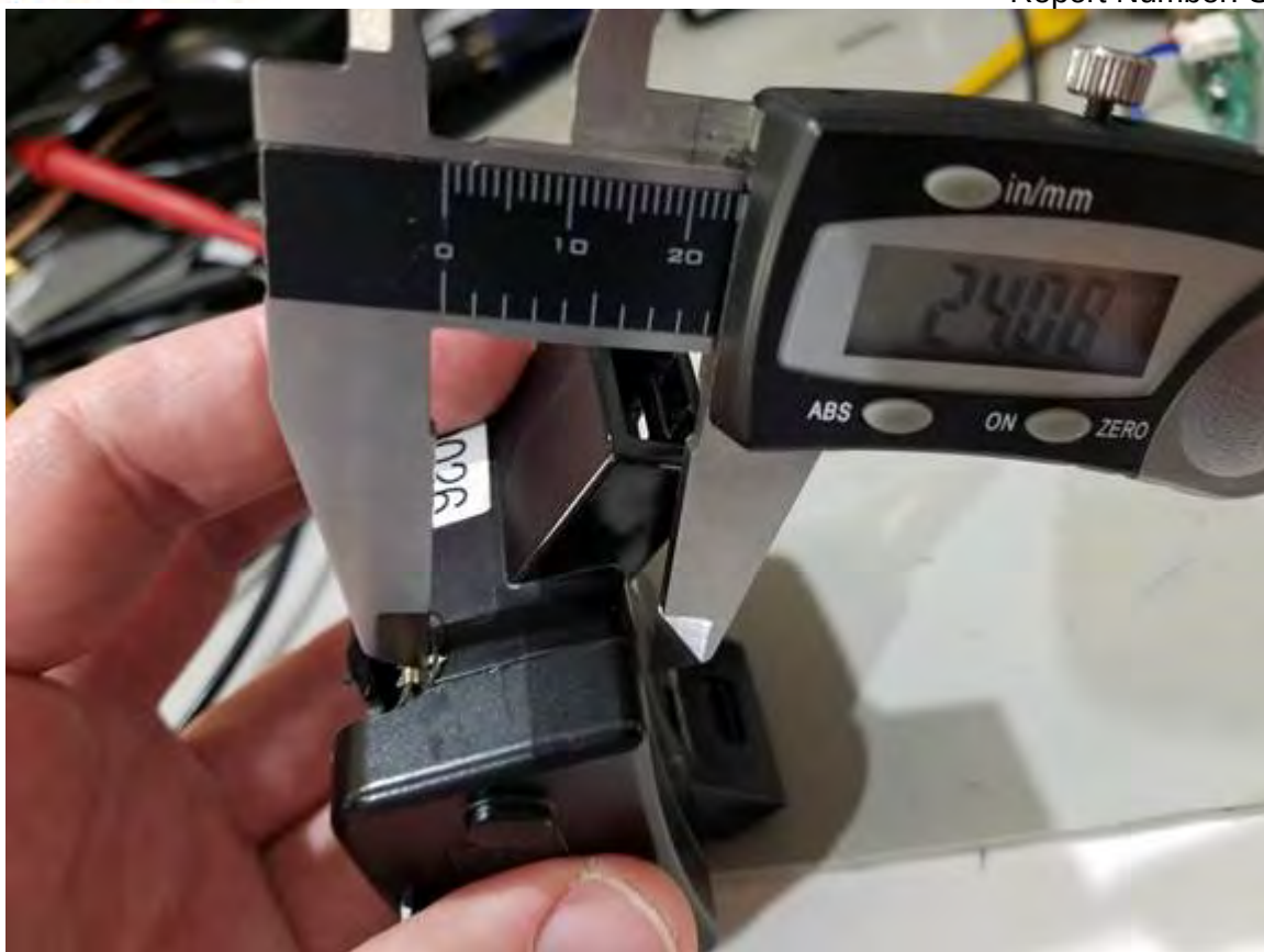
Distance of the Antenna from the User from the Back Shown on the Calipers
