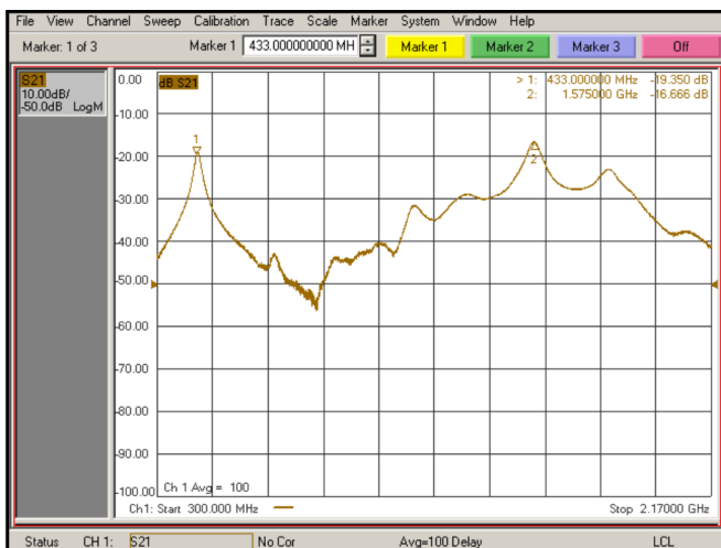
Figure 34 – Isolation between ISM antenna and GPS antenna
