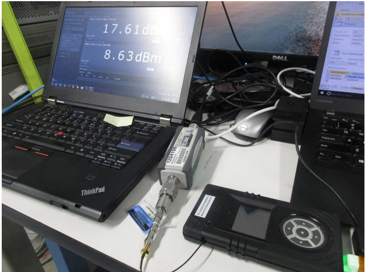
Figure 19: RF Conducted Emissions
