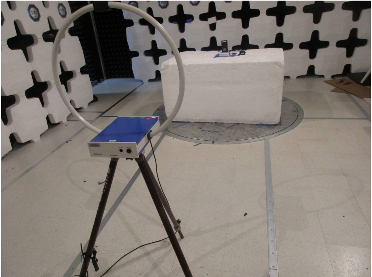
Figure 13: Radiated Emissions – Front View – Below 30 MHz – EUT Upright
