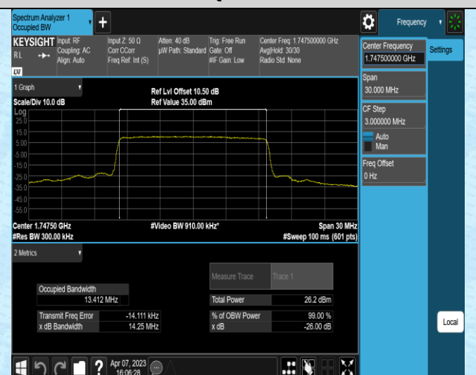
Band4-15MHz-16QAM-20025-27RB#48
