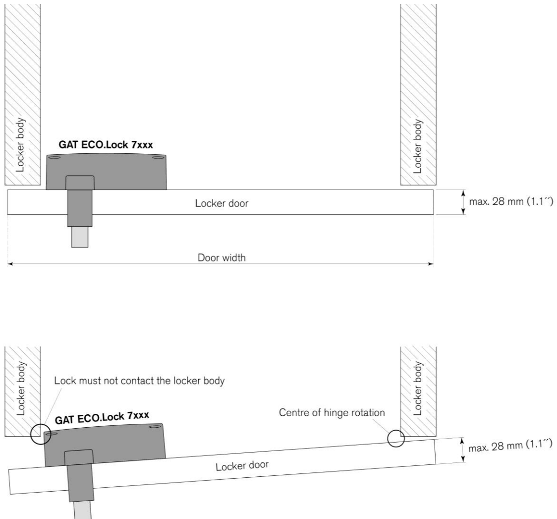
Figure 3.1 – Width and thickness of the locker door
