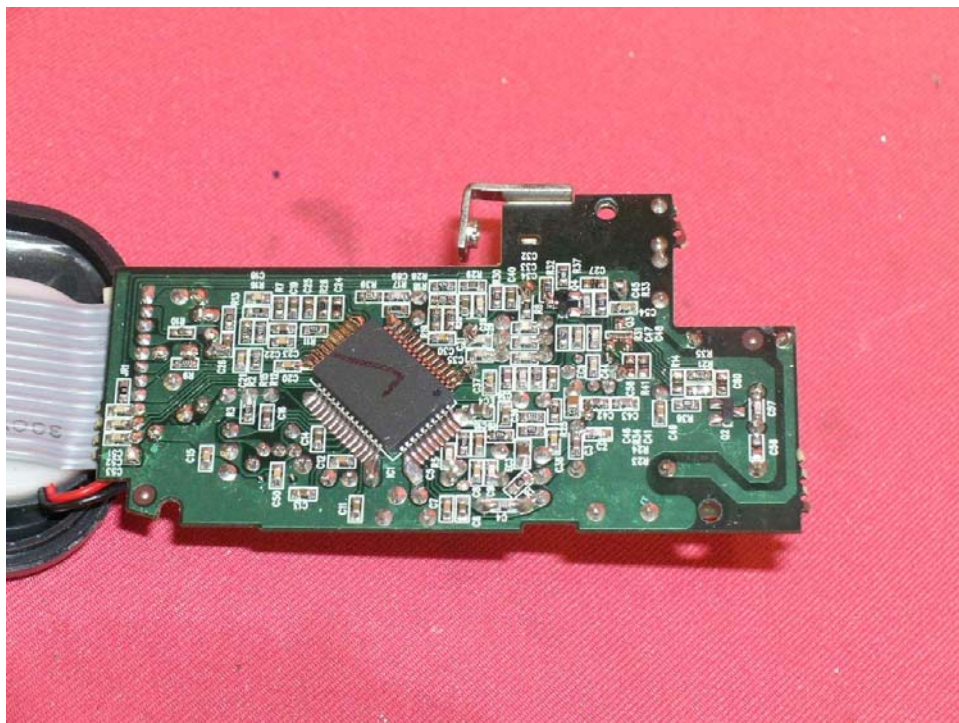
Handset Oscillator PCB solder side
