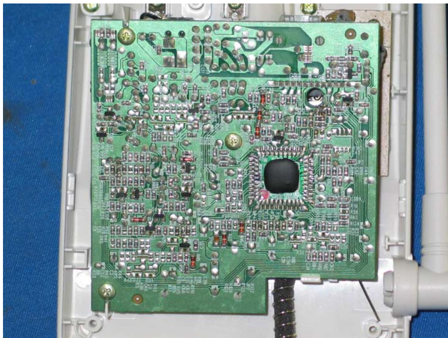
Base Unit Main PCB solder side
