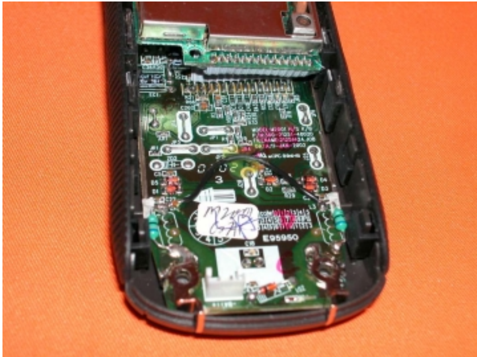
Handset Main PCB comp side (View 2)
