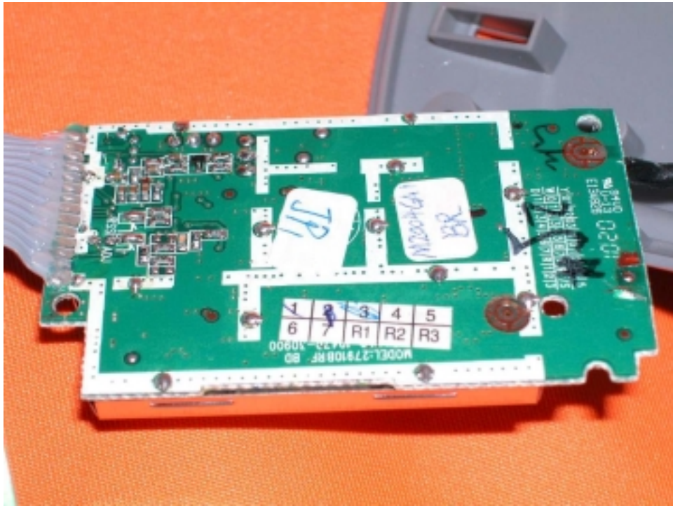
Base Oscillator PCB solder side
