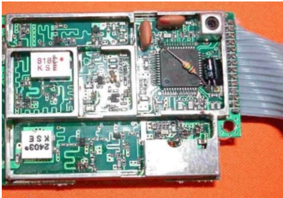
Base Oscillator PCB comp side (View 2)
