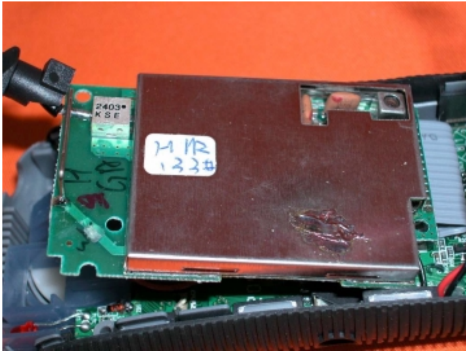
Handset Oscillator PCB comp side (View 1)
