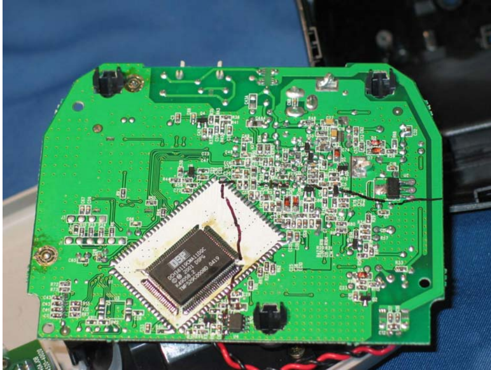
Base Main PCB solder side
