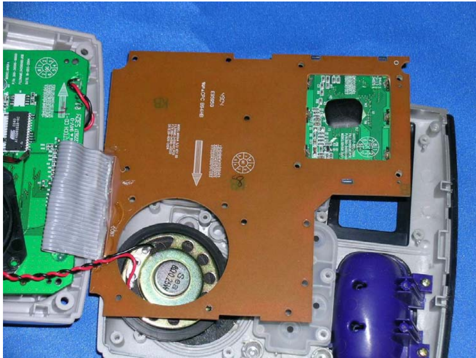
Base TAD and keypad PCB rear side
