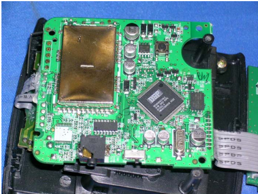
Cell Dock Main PCB comp side
