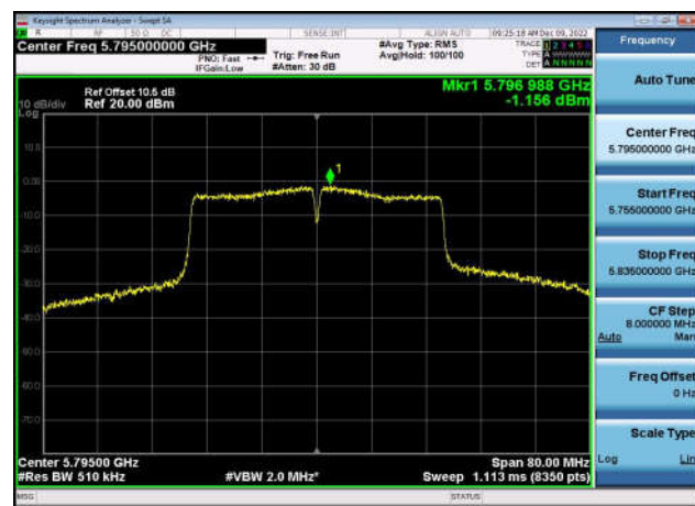
U-NII-3 Power spectral density-802.11 a(20MHz),5785MHz,Ant1
