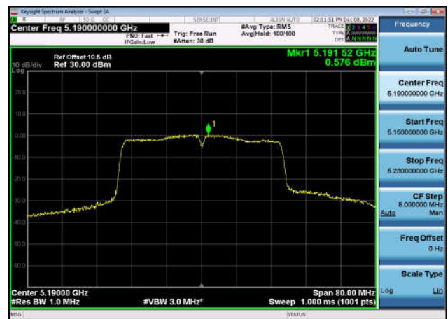
U-NII-1 Power spectral density-802.11 a(20MHz),5180MHz,Ant1
