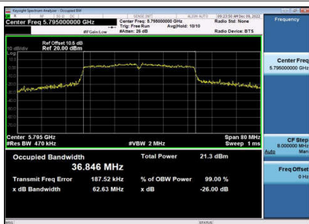
U-NII-3 26dB & 99% Bandwidth-802.11a(20MHz) ,5785MHz,Ant1
