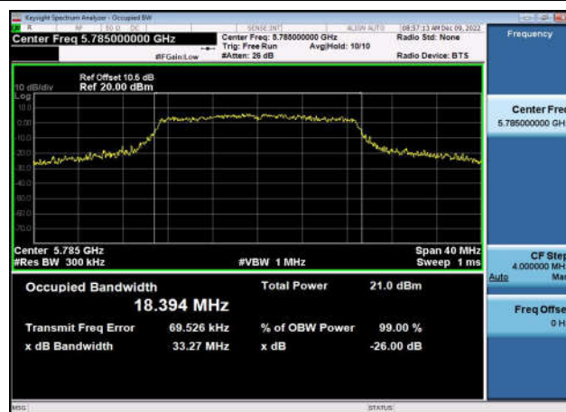
U-NII-3 26dB & 99% Bandwidth-802.11n(40MHz),5755MHz,Ant1
