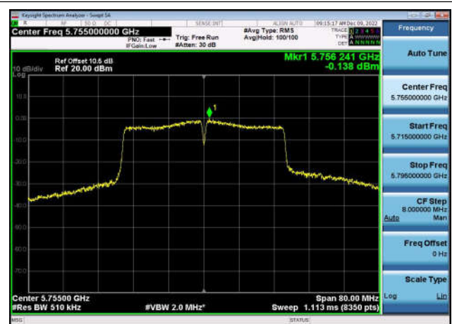
U-NII-3 Power spectral density-802.11 n(40MHz),5755MHz,Ant1
