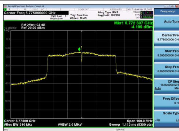
U-NII-3 Power spectral density-802.11 ac(80MHz),5775MHz,Ant1
