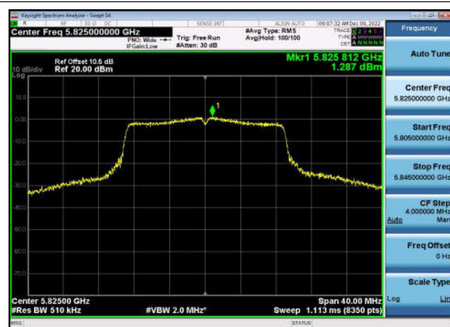
U-NII-3 Power spectral density-802.11 n(20MHz),5825MHz,Ant1
