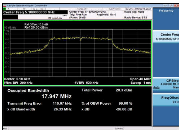
U-NII-1 26dB & 99% Bandwidth-802.11ac(20MHz) ,5240MHz,Ant1
