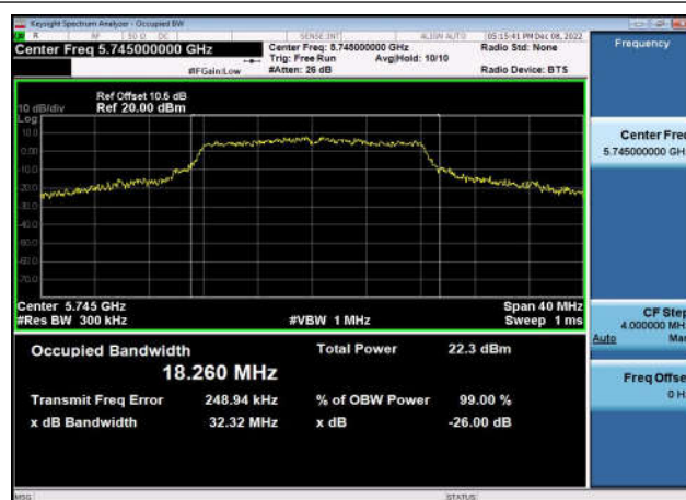
U-NII-3 26dB & 99% Bandwidth-802.11a(20MHz) ,5825MHz,Ant1
