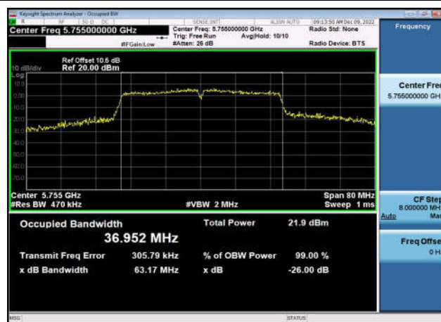
U-NII-3 26dB & 99% Bandwidth-802.11n(40MHz),5755MHz,Ant1
