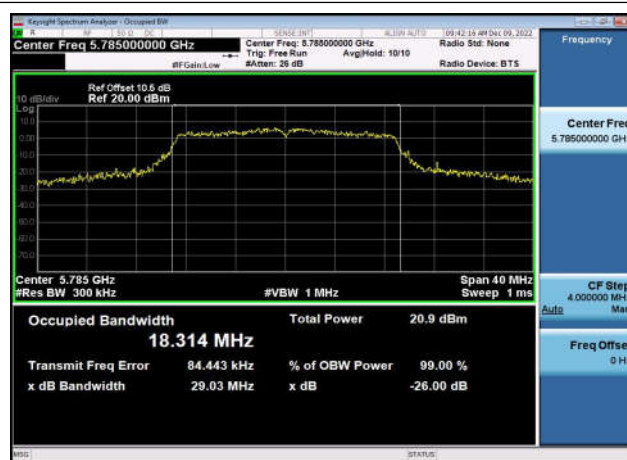
U-NII-3 26dB & 99% Bandwidth-802.11ac(20MHz) ,5785MHz,Ant1
