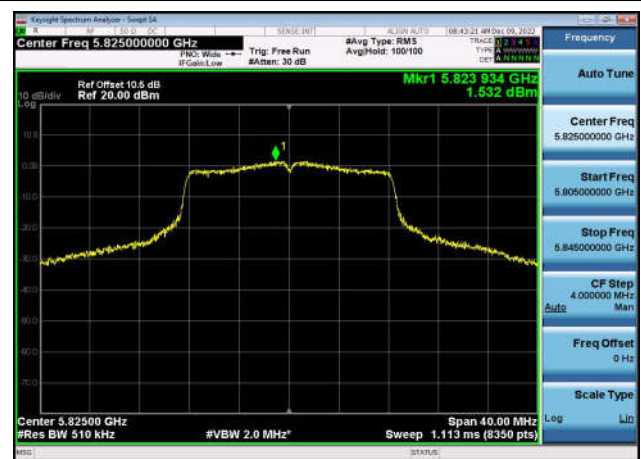
U-NII-3 Power spectral density-802.11 ac(20MHz),5785MHz,Ant1
