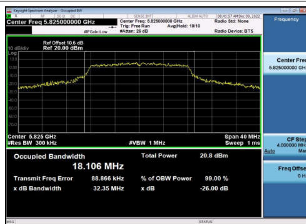
U-NII-3 26dB & 99% Bandwidth-802.11ac(20MHz) ,5785MHz,Ant1
