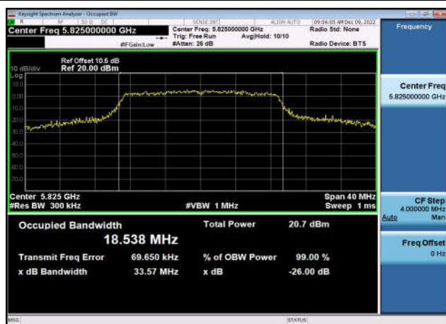
U-NII-3 26dB & 99% Bandwidth-802.11n(20MHz),5825MHz,Ant1
