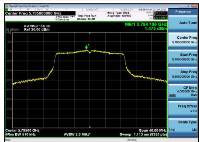
U-NII-3 Power spectral density-802.11 n(40MHz),5755MHz,Ant1
