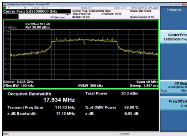
U-NII-3 6dB Bandwidth-802.11n(40MHz) ,5795MHz,Ant1
