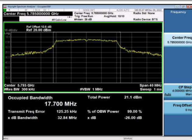
U-NII-3 26dB & 99% Bandwidth-802.11ac(20MHz) ,5745MHz,Ant1
