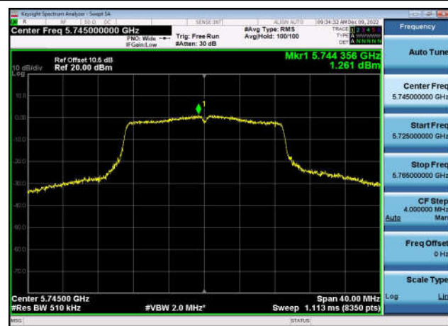
U-NII-3 Power spectral density-802.11 ac(20MHz),5745MHz,Ant1
