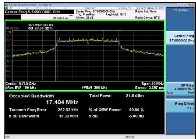
U-NII-3 6dB Bandwidth-802.11a(20MHz) ,5745MHz,Ant1
