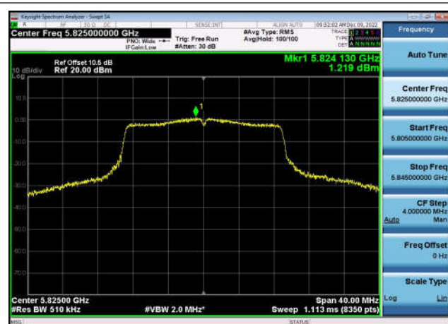
U-NII-3 Power spectral density-802.11 ac(40MHz),5795MHz,Ant1
