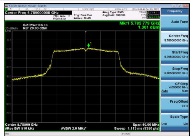
U-NII-3 Power spectral density-802.11 ac(20MHz),5785MHz,Ant1
