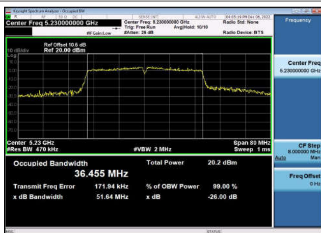
U-NII-3 26dB & 99% Bandwidth-802.11n(20MHz),5745MHz,Ant1
