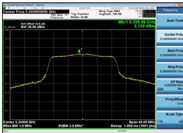
U-NII-1 Power spectral density-802.11 n(40MHz),5230MHz,Ant1
