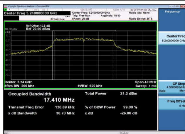
U-NII-1 26dB & 99% Bandwidth-802.11ac(20MHz) ,5220MHz,Ant1
