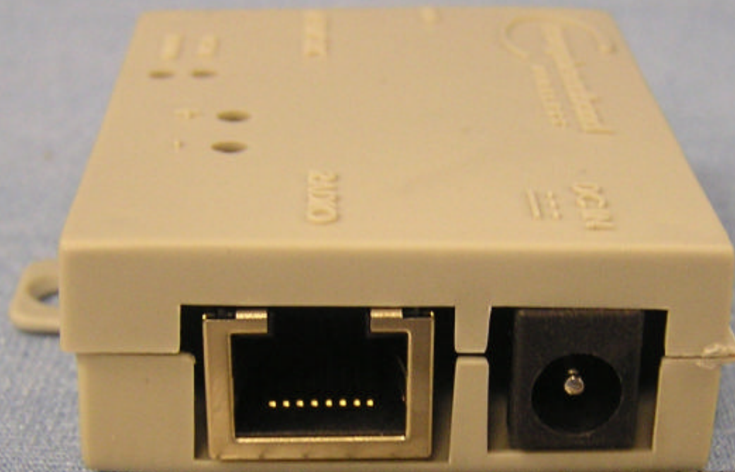
J-Box Port View
