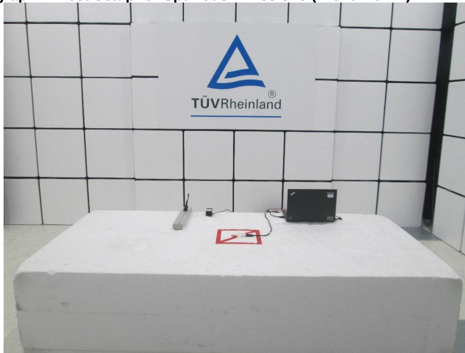
Photograph 2: Test Setup for Spurious Emissions (Front View 2)
