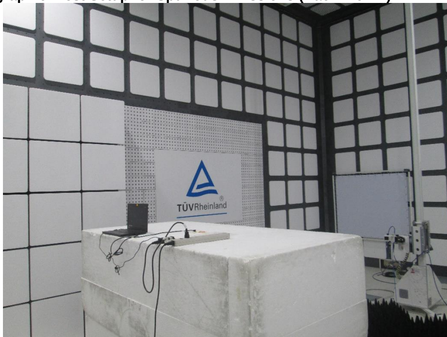
Photograph 6: Test Setup for Spurious Emissions (Back View 4)
