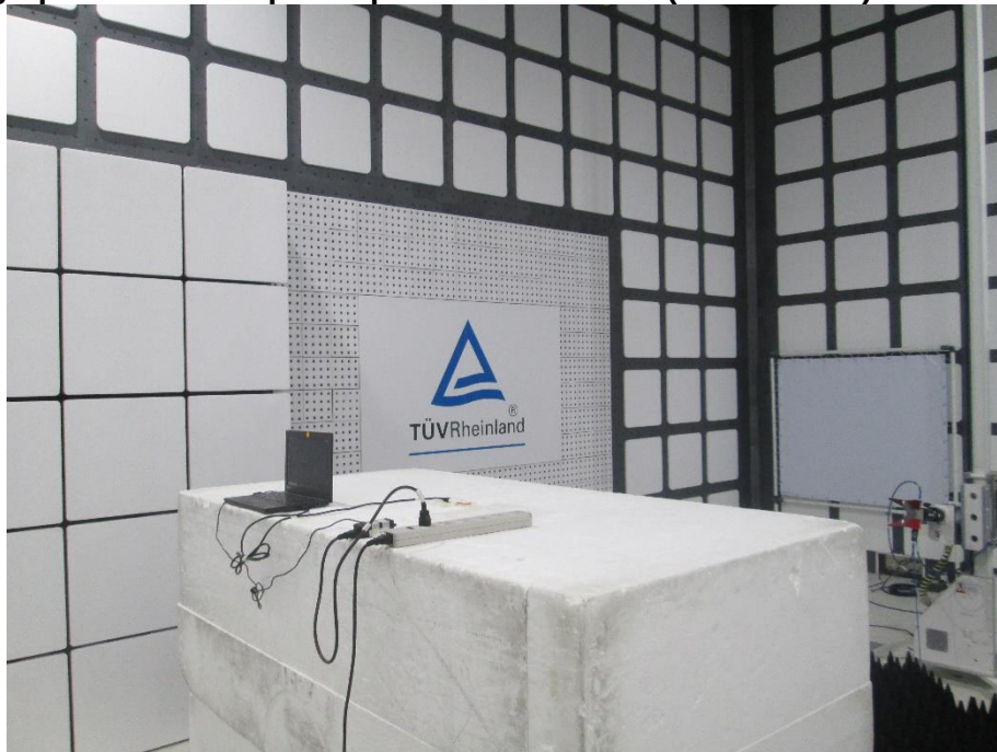
Photograph 6: Test Setup for Spurious Emissions (Back View 4)
