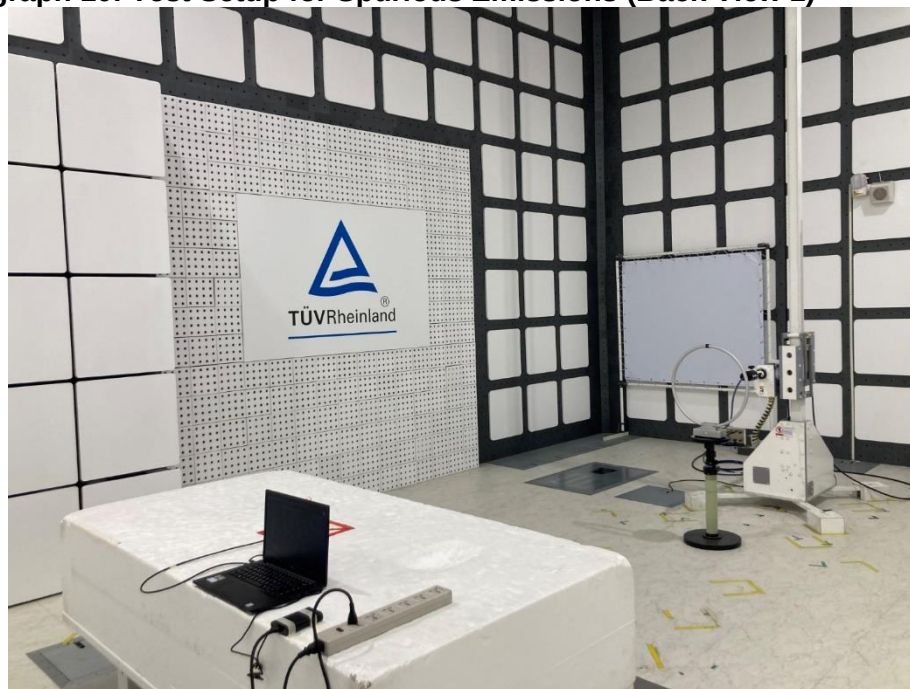
Photograph 10: Test Setup for Spurious Emissions (Back View 1)
