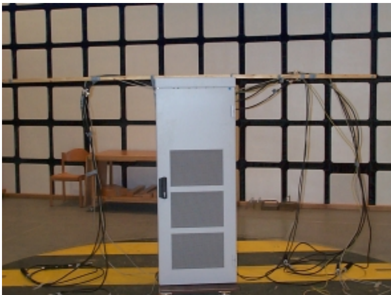
Fig. 31 -- Photograph of the anechoic chamber with the EUT (configuration A).
