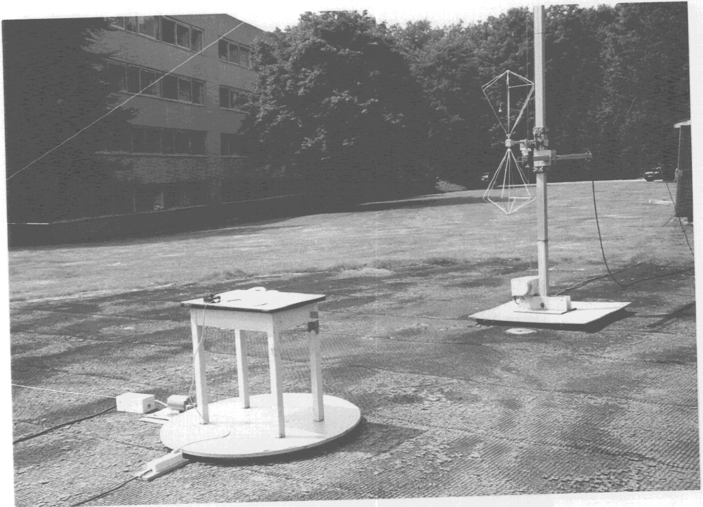
5.2 Radiated emission measurement setup at the OATS
