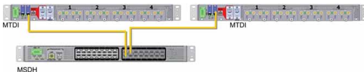
Figure 4-7. Example of MSDH to MTDI Connections
