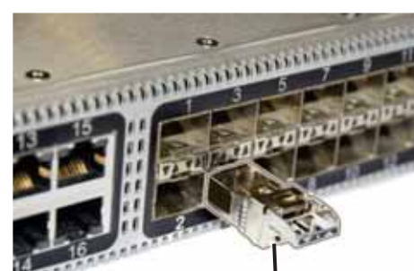
Cobham Wireless SFP+ Install in MSDH BOTTOM CPRI row (Label facing DOWN)
