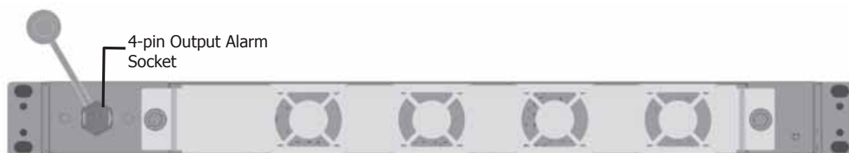
Figure 4-9 MSDH Public Safety Output Alarm Connections
