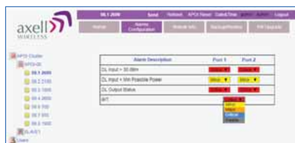
Figure 6-34. External Alarms Definitions
