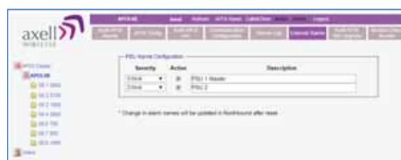
Figure 6-33. External Alarms Definitions
