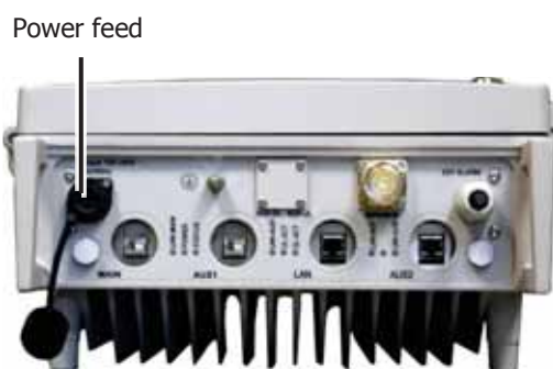
Figure 5-31. Front Panel Example Showing Location of Power Connector
