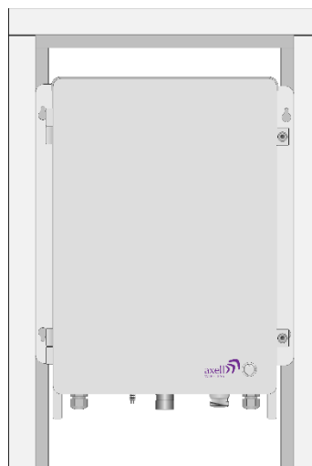
Figure 4-5: Rack-mount Repeater position
