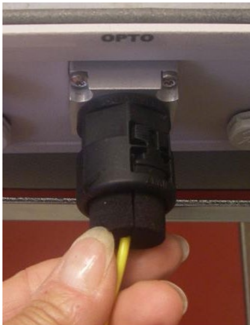
Figure 4-20: Adjust F/O cable length
