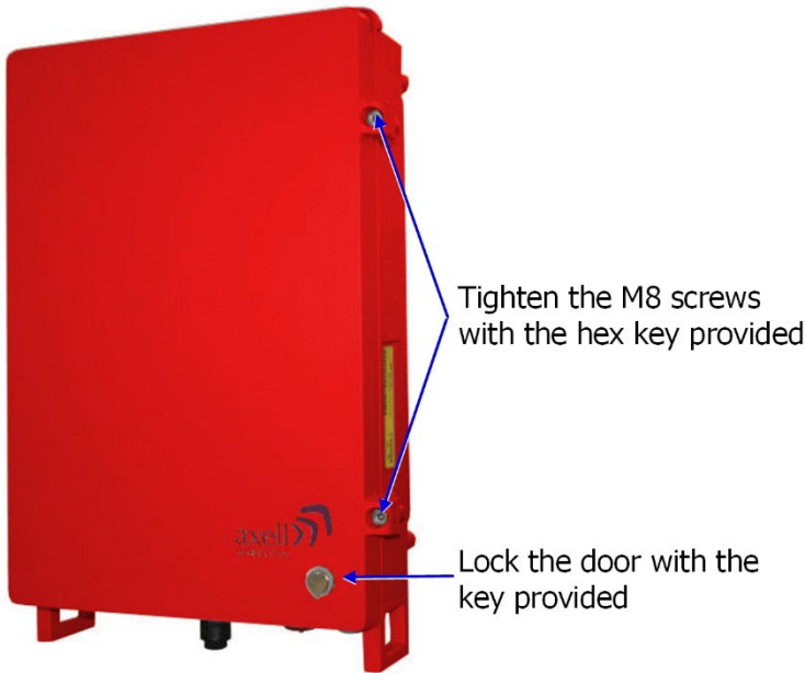
Figure 3-4: Securing the Repeater
