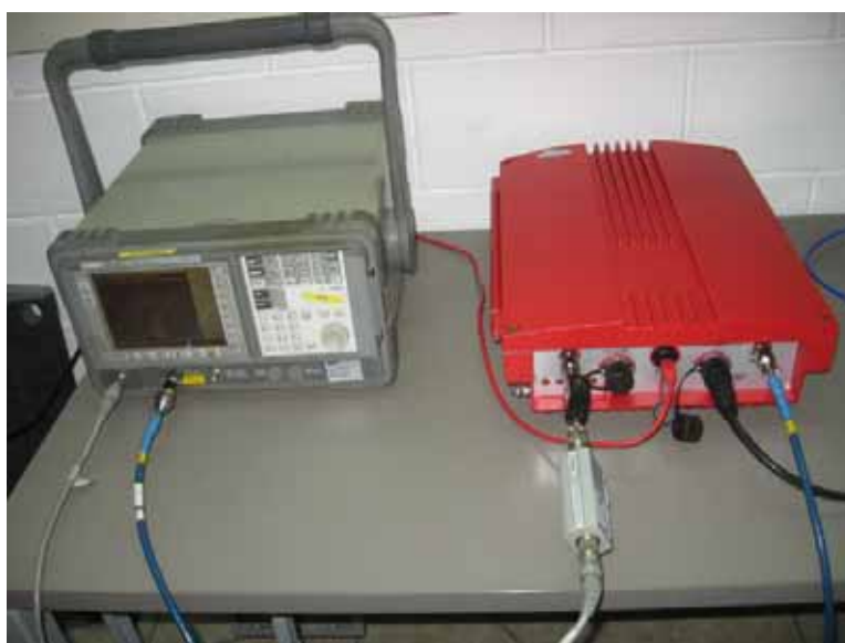
Photograph 7.8.1 Noise figure test setup
