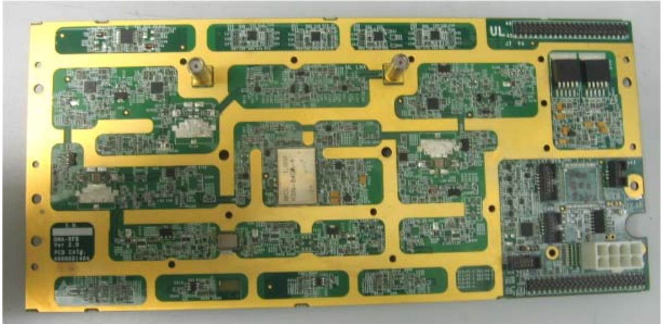
Photograph No.16 RF PCB front view
