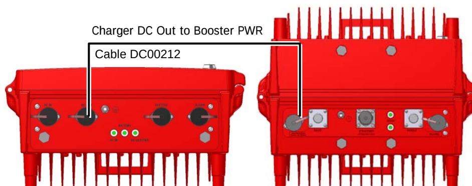
Figure 3-19 Battery Charger to Booster Power Connections
